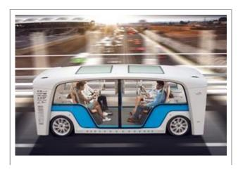
cameras, radar, LIDAR and a host of other safety-related sensor systems. It can be a challenge to integrate these into a vehicle in a manner that optimizes performance while maintaining a clean design aesthetic. Gentex dimmable glass panels, or sensor shrouds, darken on-demand or automatically according to sensor function. On Snap, they work to conceal and optimize the operation of forward-facing cameras, optical systems, communication components, and the autonomous sensor farm.
