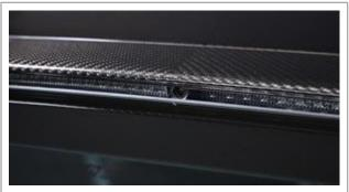
The video feed from this roof-mounted camera is combined with the feeds from the exterior-mirror-integrated cameras and displayed in multiple composite views in the Gentex Full Display Mirror (FDM).
