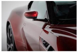
This Aston Martin DBS Superleggera features a hybrid camera monitoring system (CMS) that uses three cameras to provide a comprehensive view of the sides and rear of the vehicle. Side-view cameras are discretely housed in each of the vehicle's exterior mirrors; their video feeds are combined with that of a roof-mounted camera and displayed together in multiple composite views that are streamed to the driver via a rear-view mirror-integrated display inside the cockpit.
