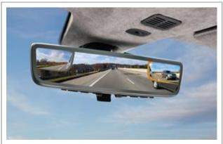
Central to the hybrid CMS solution is the Gentex rearview-mirror-integrated display known as a Full Display Mirror (FDM). The FDM can function as either a standard auto-dimming rearview mirror or as an
