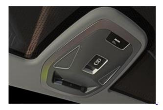
The core of Guardian's technology is an infrared-sensitive, high-resolution camera that combines machine vision, depth perception, and micro-vibration detection. This proprietary sensor configuration allows the system to not only monitor the driver, but also the entire vehicle cabin and all its objects and occupants.
