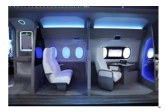
Gentex's aircraft mockup features fully functioning dimmable windows and cabin partitions; passenger smart-lighting that automatically optimizes illumination for various in-flight activities like reading, dining, or computer work; biometric systems for personalizing the in-flight experience; and in-cabin particulate and chemical sensors for monitoring cabin air quality.
