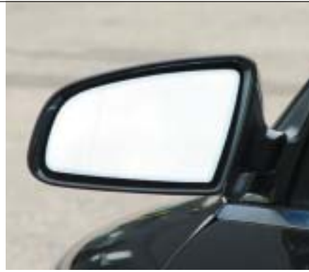
Gentex's "chrome ring" mirror eliminates the need for a plastic bezel on the exterior mirror glass sub-assembly, increasing the mirror's field-of-view and enhancing its appearance.
