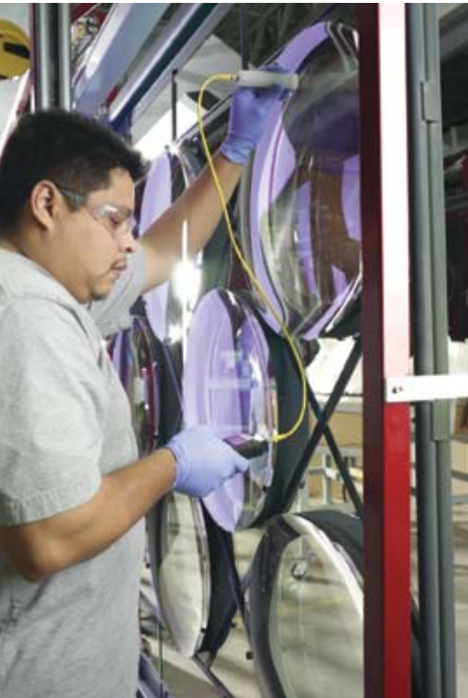
Testing the electrical resistance of exterior mirror glass coating on one of Gentex's in-house coaters
