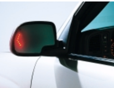
LEDs are combined into exterior mirrors to form the world's first automatic-dimming mirrors with turn-signal indicators.
