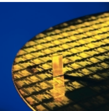
ABOVE: Gentex's Active Light Sensors and SmartBeam cameras are actually semiconductor chips, which are manufactured on silicon wafers, and utilize the same methods used to make computer chips. Gentex recently initiated prototype production on its microelectronics line where these chips are designed, tested and packaged.
