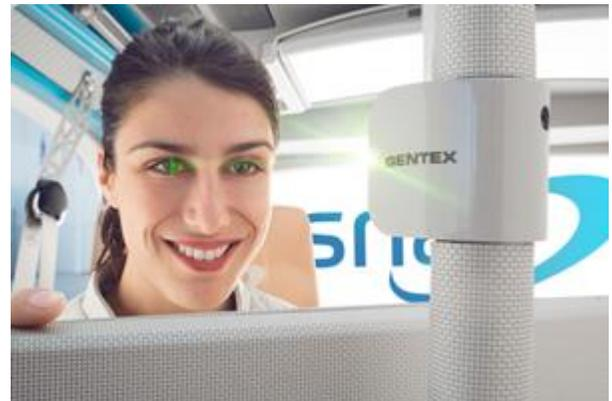
For Snap, Gentex developed a vehicle-based biometric ID module that authenticates the passengers and delivers customized security, comfort and convenience features. The system consists of a small module that houses near-infrared emitters, an iris-scanning camera, and system-level intelligence.
