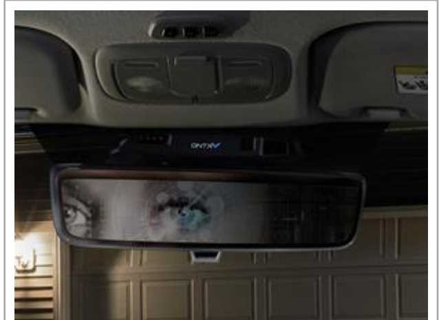
Gentex's new vehicle-based biometric identification system authenticates the driver with an iris scan and delivers customized security, comfort and convenience features. The system can also be used to help secure and enhance vehicle-to-home automation services as well as vehicle-to-infrastructure transactions.
