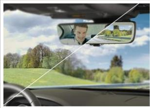
Gentex's Full Display Mirror is an intelligent rear-vision system that uses a custom camera and mirror-integrated video display to optimize a vehicle's rearward view. The system captures video from a rearward-facing camera and streams it to a unique mirror-integrated LCD that provides the driver with an unobstructed, panoramic view behind the vehicle. This year at SEMA, Gentex is demonstrating an FDM capable of toggling between two different camera inputs.
