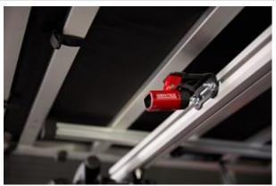
Gentex has developed a wired, detachable auxiliary camera that can affix to a truck tailgate, camper or trailer, which could provide rear vision when the primary vehicle-integrated camera is blocked.
