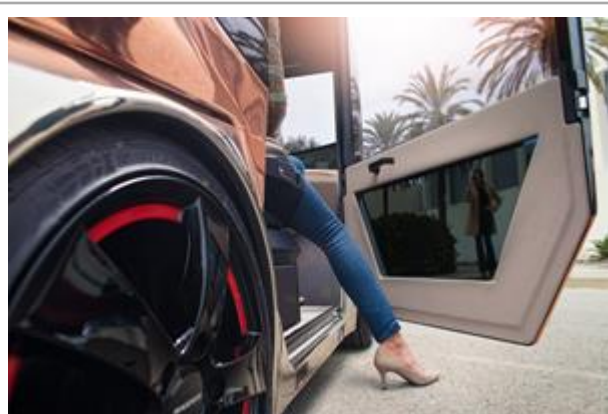
To help ensure passenger privacy, Gentex provided microSNAP with dimmable glass panels that darken on demand or in conjunction with sensor function. They can even assist the climate control system in maintaining a consistent temperature by darkening according to temperature and sun load sensors.
