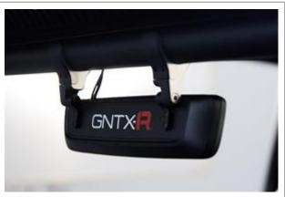
The Gentex R-Series Full Display Mirror is a digital rear vision system specifically designed for professional racecar teams. It includes a high-performance, mirror-integrated LCD and rearward-facing camera module to provide a vehicle's rear view.
