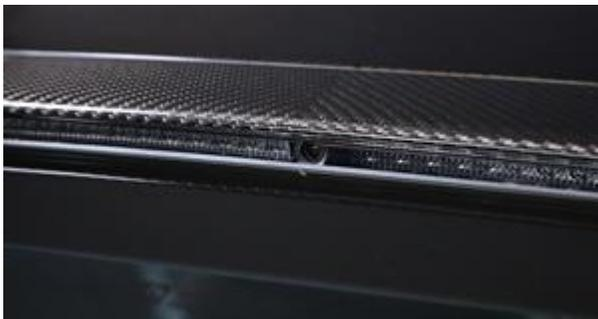
The video feed from this roof-mounted camera is combined with the feeds from the exterior-mirror-integrated cameras and displayed in multiple composite views in the Gentex Full Display Mirror (FDM).
