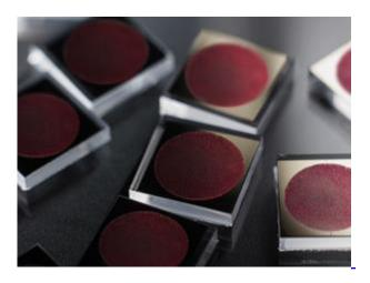
A nanofiber sensor chip contains nanofibers approximately one thousand times smaller than a human hair. Their large porous surface area provides optimal absorption of chemical vapors that can result in sensitivity in the parts per billion range for most target compounds and in the parts per trillion range for some chemicals.
