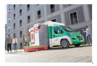
Rinspeed's CitySnap is a proof-of-concept delivery vehicle designed to highlight innovative, sustainable, and efficient urban delivery. Central to the concept are mobile locker units that are transported, delivered and "hot swapped" to parcel stations throughout a city.
