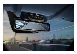
LCV's typically have poor rear vision. Consequently, LCV manufacturers are turning to Gentex's Full Display Mirror, an intelligent rear-vision system that uses a custom camera and mirror-integrated video display to optimize a vehicle's rearward view.
