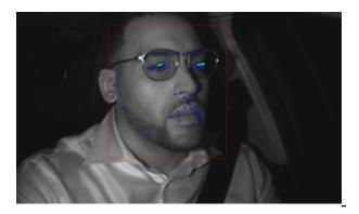
The Gentex driver and cabin monitoring system tracks the driver's head pose, eye gaze, and other vision-based metrics to determine driver distraction, drowsiness, and readiness for return of manual control in semi-autonomous vehicles.
