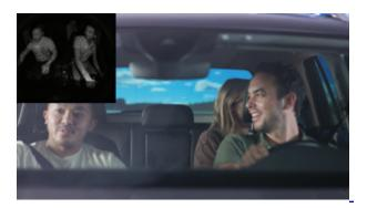
Gentex's mirror-integrated DMS tracks driver head pose, eye gaze, and other metrics to determine distraction, drowsiness, sudden sickness, and return of manual control in semi-autonomous vehicles. The system can expand to include 2D and structured-light-based 3D cabin monitoring for detecting passengers, behavior, objects, and even presence of life.
