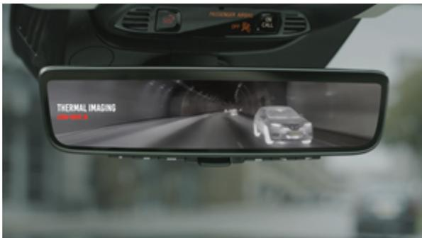
Gentex and ADASKY are partnering to integrate thermal imaging in a Gentex Full Display Mirror (FDM), the industry's leading digital rearview mirror. The inclusion of a rearward-facing thermal camera in an FDM system could dramatically improve the driver's ability to monitor the rearward scene during nighttime driving and help identify potential hazards while reversing.
