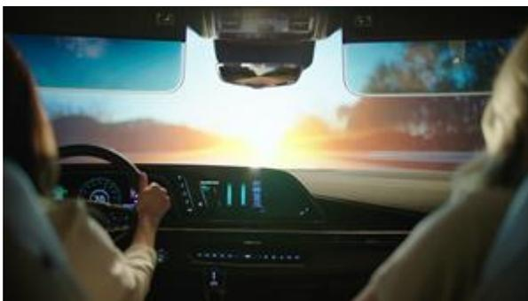
Gentex's innovative sun visors feature clear, dimmable panels that automatically adjust to prevent sunlight glare. The latest version incorporates a switchable reflective surface, allowing them to not only eliminate sunlight glare, but also function as vanity mirrors.
