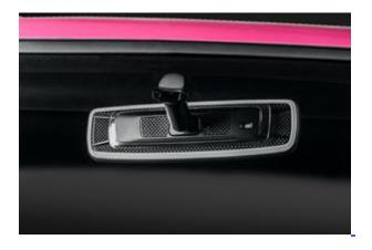
INFECTED features a custom, high-tech, carbon-fiber mirror from Gentex. It uses cameras to detect headlight glare and darken automatically to protect driver vision.
