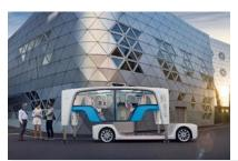
Rinspeed's Snap concept vehicle consists of two parts: an autonomously driven chassis, or "skateboard," that docks with various customizable passenger safety cells, or "pods." Separating the vehicle into two components allows the autonomous skateboard to operate 24/7, serving multiple customers throughout the day. The chassis are replaced as mechanical components wear out and IT components reach obsolescence. The more durable and versatile passenger pods would live on and be personalized for
