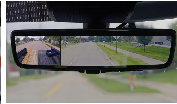
BED CAM VIEW Shows pickup bed and rearward view
