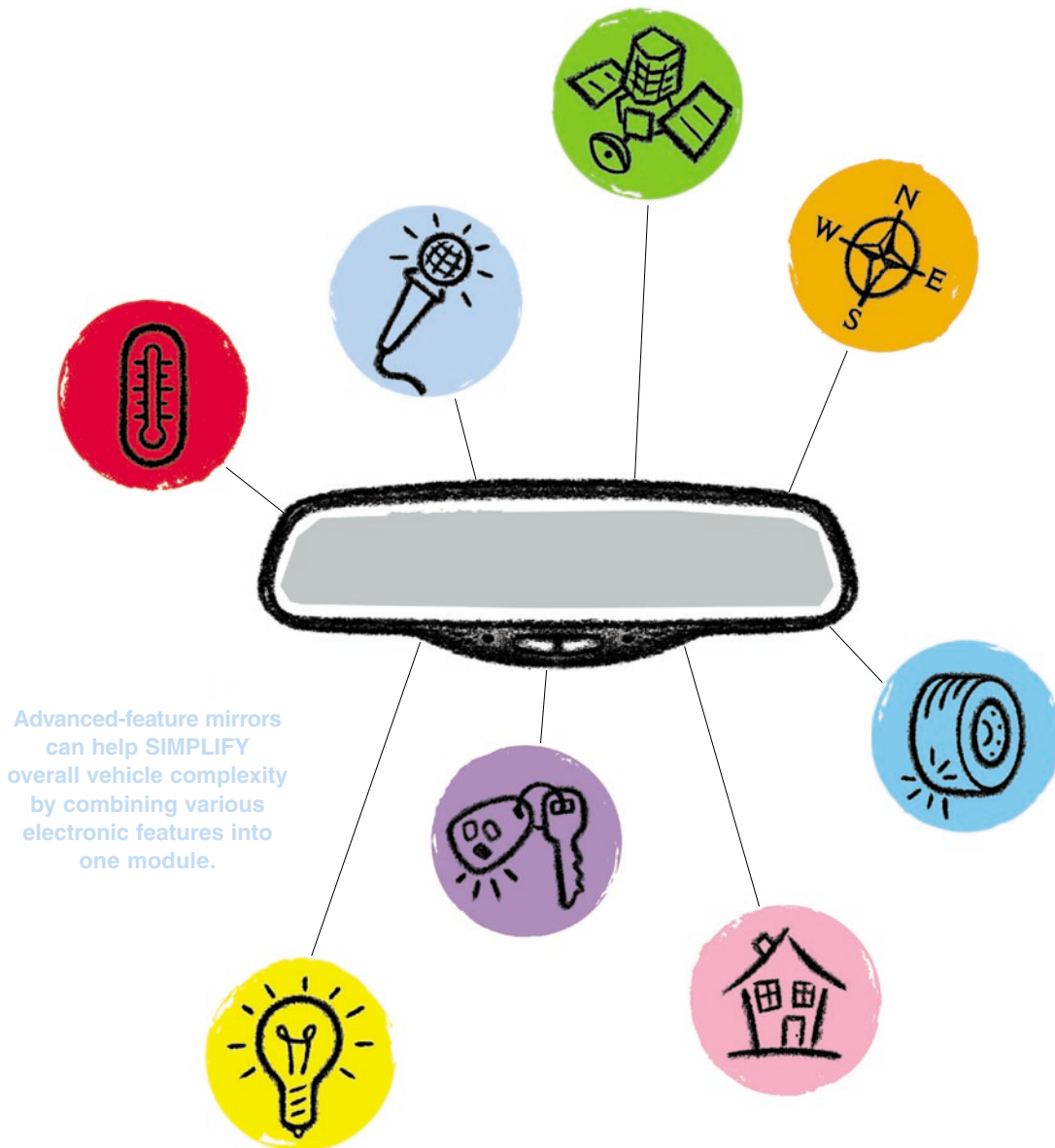
Clockwise from top left: Temperature display, Microphone, GPS Components, Compass display, Low-tire-pressure monitoring, Remote home/garage controls, Remote keyless entry, LED map lamps
